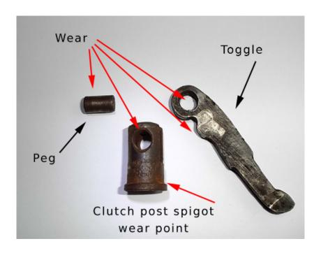
Having briefed yourself on the overall picture with the above bed - time reading and learnt how to refurbish the fulcrum points on the clutch plate, where the toggle arms pivot, here are the "extra" thoughts!
