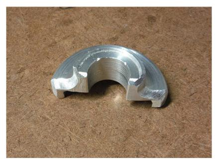
Repair section, cut, chamfered and ready to weld
