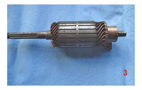
Carefully clean off the copper deposits on the end cover and reach down between the field windings on the main body. There are strong springs to hold the brushes in contact with the armature; check that these are in good order and
