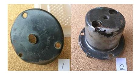
The main issue to look for is the thin brass switch cover plate wears (pic1) this results in the copper contacts of the switch not meeting squarely. The switch button copper contact becomes damaged giving a poor electrical connection with possible overheating or even a short circuit. Picture 2 shows one that has had this event and melted a hole in the steel switch body!
