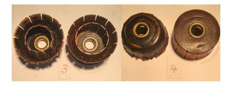
Remove the double nuts, flat and spring washers and outside insulation washer. Tap out the two half round triangular copper contacts, carefully remove the thin insulating strip wound inside the switch body sides which is .023 thick followed by the insulator in the bottom of the switch body.
