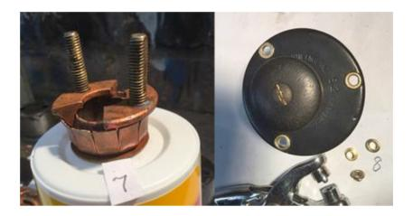
The left hand contact in my pictures has been so hot it melted, copper melts at 1084°C and is now too soft to be any use other than to flatten it out for a pattern to make a new one. No spare contacts are available as far as I know. The worn switch cover can be recovered by soldering a flat washer inside to cover the elongated hole.
