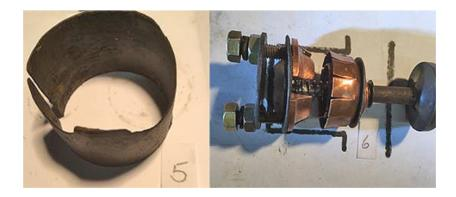
If your switch contact is like the one on the right of pic3 leave as an assembly on the button shaft and give it a good clean to bright copper. If it's badly out of
