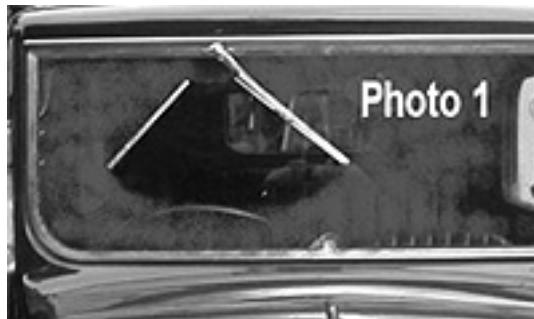
I stripped down the DW3 and reasoned that if I moved the pivot point further from the centre of the 'Gear' wheel I should be able to get more travel to the connecting arm and thus increase the swept angle of the wiper arm. I did experiment with a number of holes - *Photo 2* - in a spare gear wheel and settled on an increase of 1.7mm from the centre of the gear wheel to the new point ('A' is original, 'B' is the final hole, 'C' and 'D' are experimental holes).
